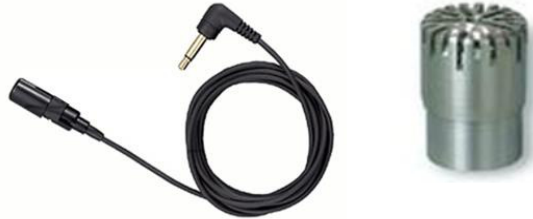
Figure 5: Example of microphones used for IE. Left: simple capacitor microphone (50 - 16000 Hz), Right: high precision microphone (4 - 20000 Hz).
