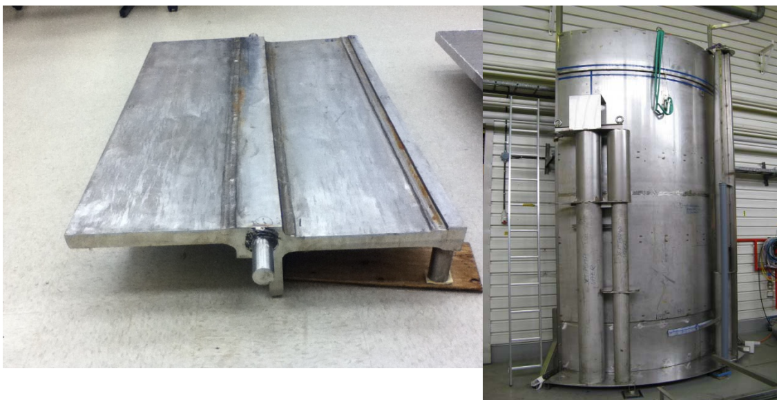
Figure 3: Qualification of core shroud inspection.
